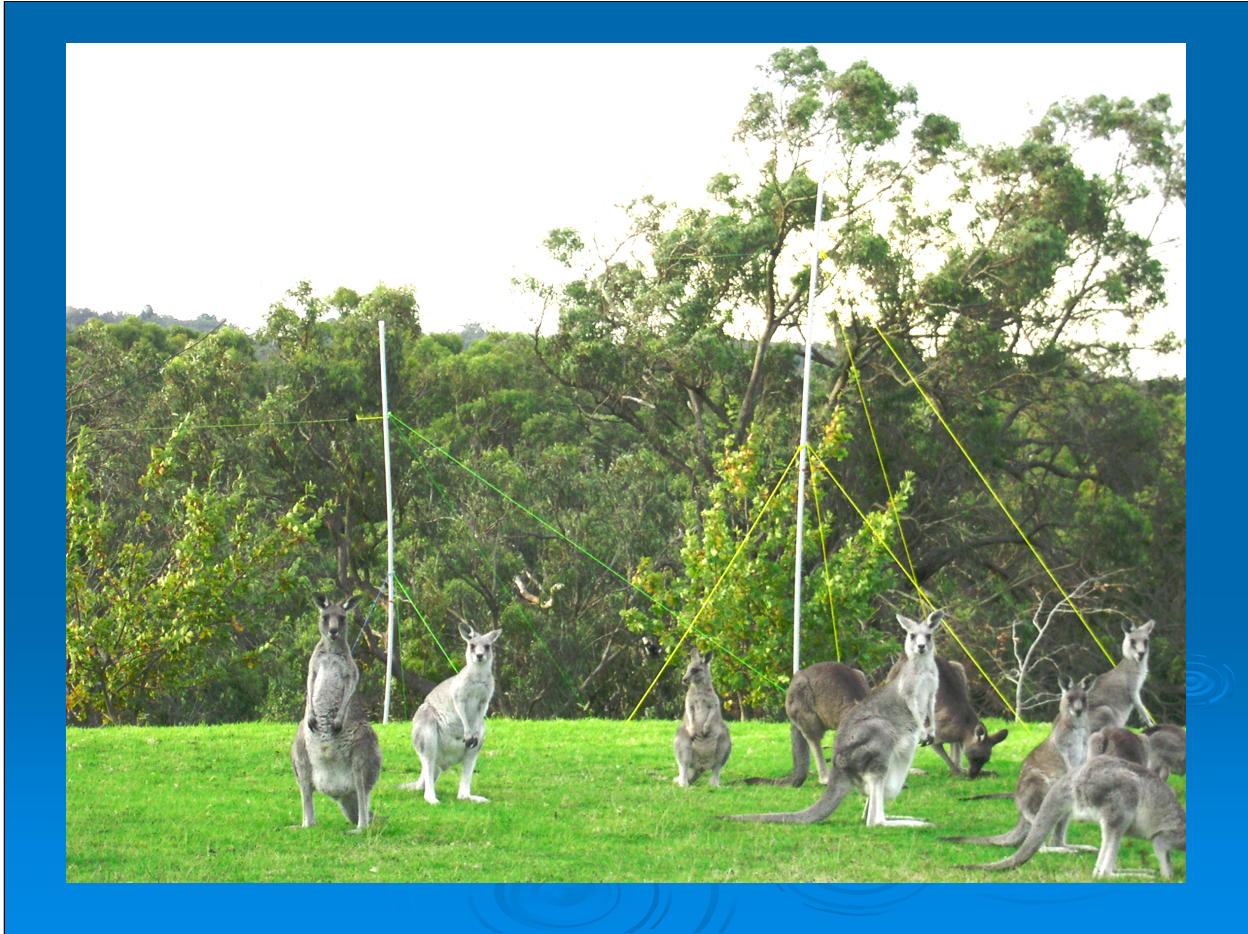
The Jove dual dipole array – easy to erect with a little help. While it is cut for 20 MHz operation it is usable with a spectrograph over as much as 4 MHz.
